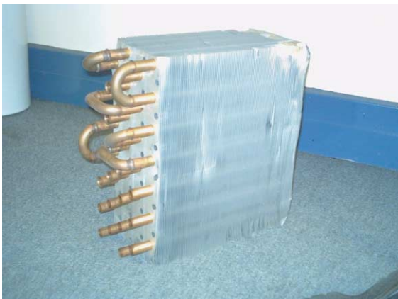
Fig. 1. Photograph of a fin exchanger block.
